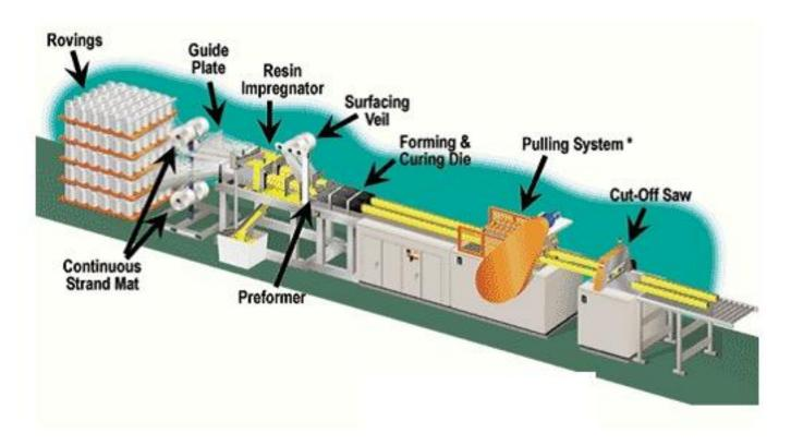
The creels position the reinforcements for subsequent feeding into the guides. The reinforcement must be located properly within the composite and this is the function of the reinforcement guides.
