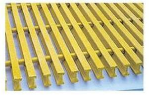
The pultruded grating provides increased load capacity with moderate levels of corrosion resistance. The components (bearing bars and cross bars) are pulled by machine to have a higher reinforcement content. Its superior load capacity is a result of the higher reinforcement to resin ratio. The pultrusion process is automated and produces a consistent, high quality finished product. Assembled from bars,
